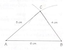
When an angle is identified by three letters, the middle letter indicates the vertex of the angle. For example, ∠A is also ∠CAB.
